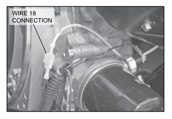
Figure 33. Wire 18 Connection 8 kW Units
